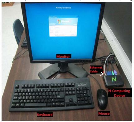
N-Computing Detailed picture with PS2 Connections
